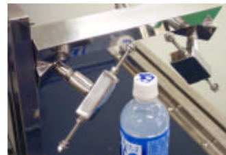
Blowing off of water before shrink wrap packing
